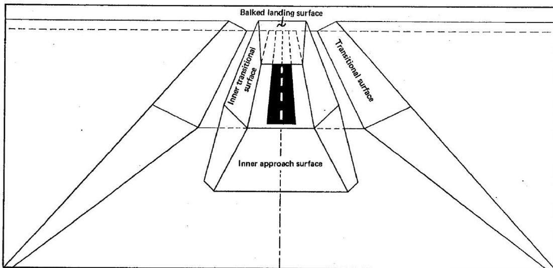
Figure 20: Obstacle free zone surfaces - 3D view
