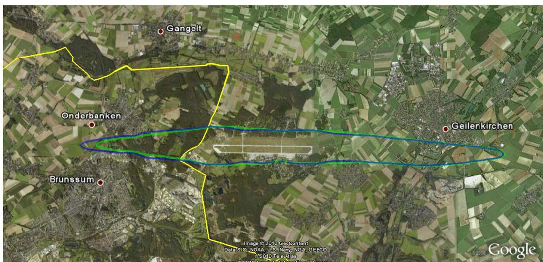
Figure 6: Comparison of 35 Ke contours for the current and with the extended runway
