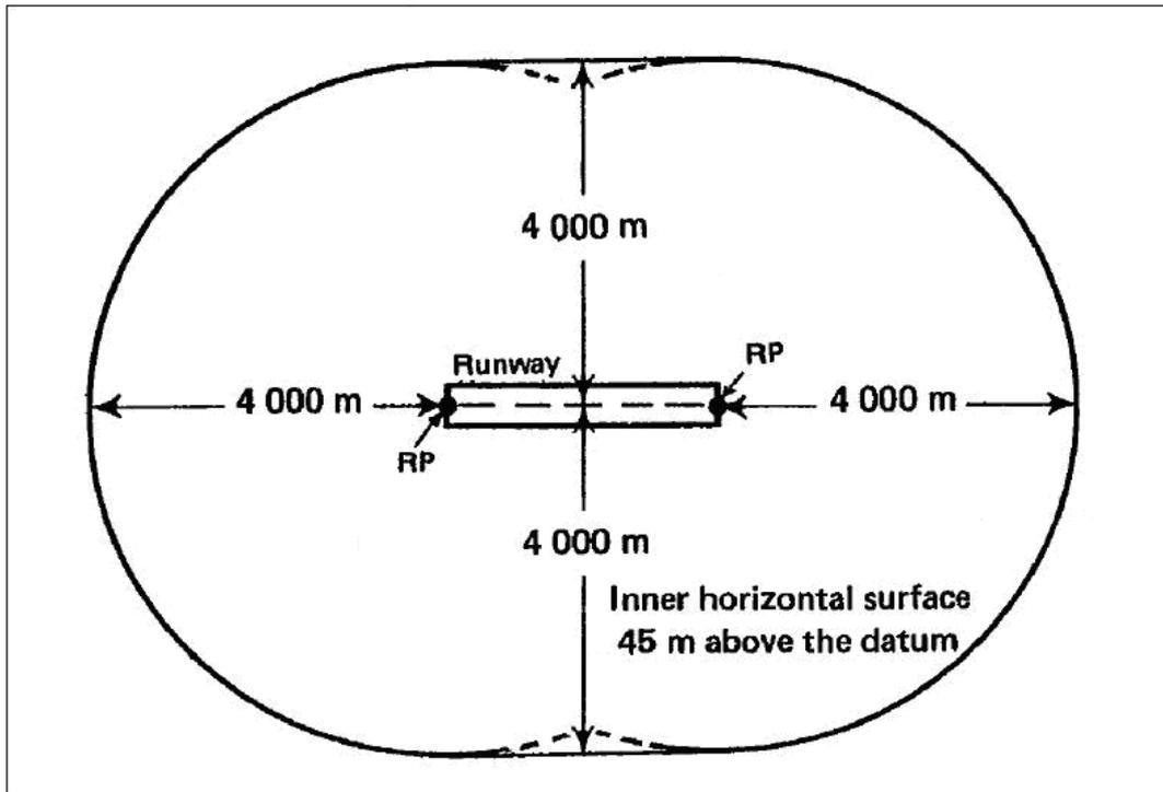
Figure 18: Inner horizontal surface for a single runway
