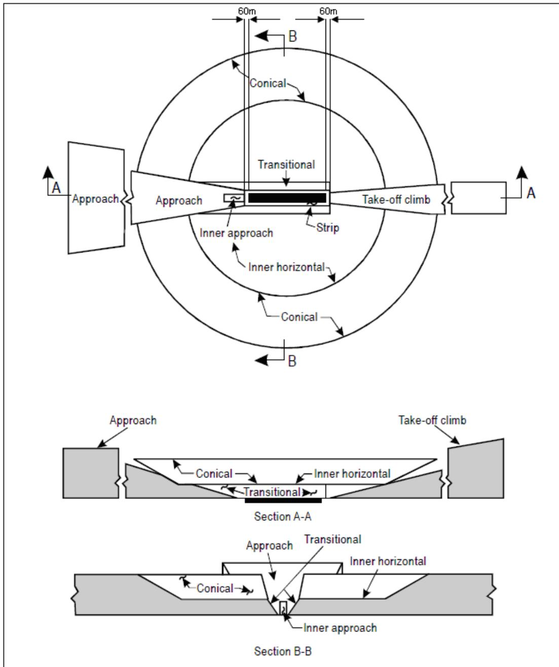
Figure 17: Obstacle limitation surfaces according to ICAO Annex 14
