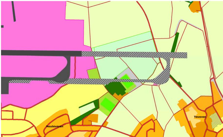
Figure 12: Detail: the extended runway crossing existing roads
