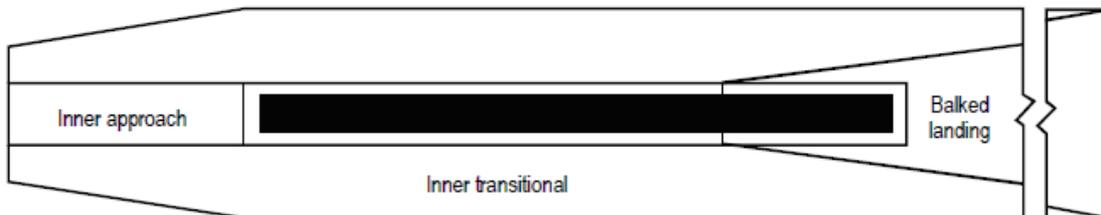
Figure 19: Obstacle free zone surfaces - inner approach, inner transitional and balked landing obstacle limitation surfaces according to ICAO Annex 14
