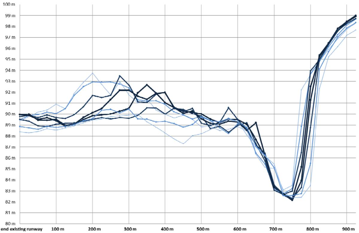
Figure 14: Height differences in the area of the runway extension: side view
