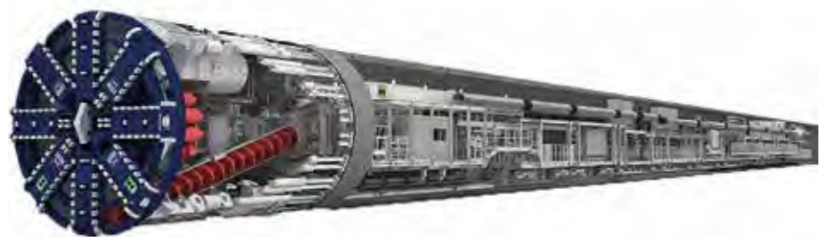
Figure 2-4: A large TBM (7.1 m diameter) used for the boring and lining of 42 km of 6.2 m diameter rail tunnels for the Crossrail system at depths of up to 40 m beneath London. The image shows how concrete tunnel liner segments are emplaced behind the cutting head as tunnelling progresses, as envisaged for the Dutch GDF tunnels (image: crossrail.co.uk).
