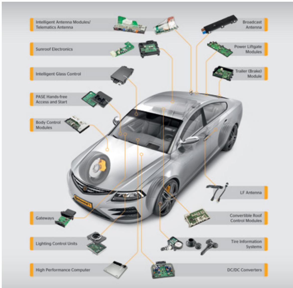
Figuur 12: Verschillende Electronic Control Units (ECU) in de auto. (Bron: Continental 98 )
