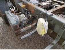
A Volvo from 2000, for Nigeria with many deficiencies: VIN unreadable, lights and battery removed, exhaust system incomplete, bumper missing, fuel tank missing, air tanks hanging loose, smooth tires
