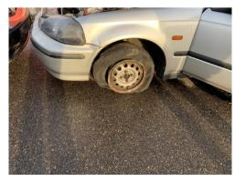
A heavily damaged car after an accident, a Nissan Micra from 2003 for Benghazi, Libya (left picture). A Honda Civic from 1996 for Lybia. The axles, wheels and tyres had several deficiencies (right picture).
