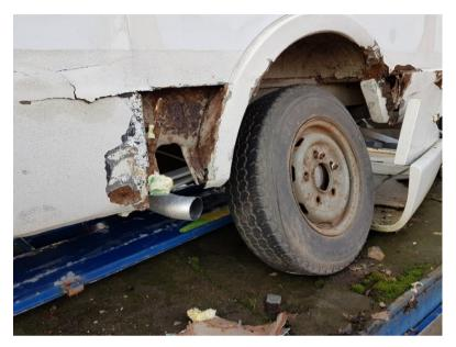
A Volkswagen bus LT3590 from 1988 for Lagos, Nigeria with many damages: left auxiliary beam 100% rust damage, shaft seriously deformed, heavy gasoline smell
