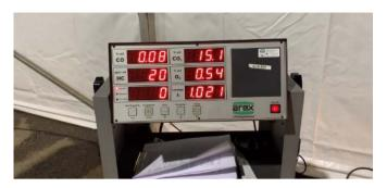
Inspection of a ten-year-old Euro 4 Hyundai for Ghana with functioning catalytic converter
