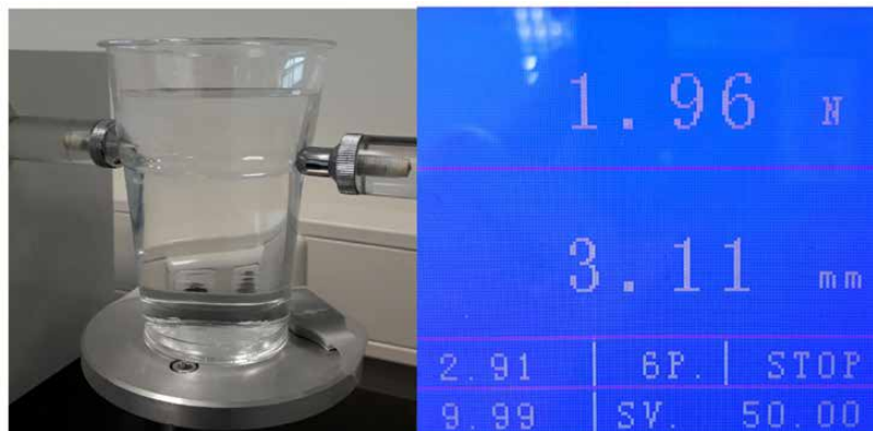
Figure 39: Cup Compression Tests instrumentation
