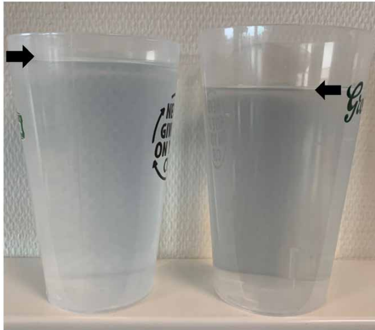
Figure 38: The 200 and 250 ml (H)PP 1 Hard Cups filled with 250 ml of water
