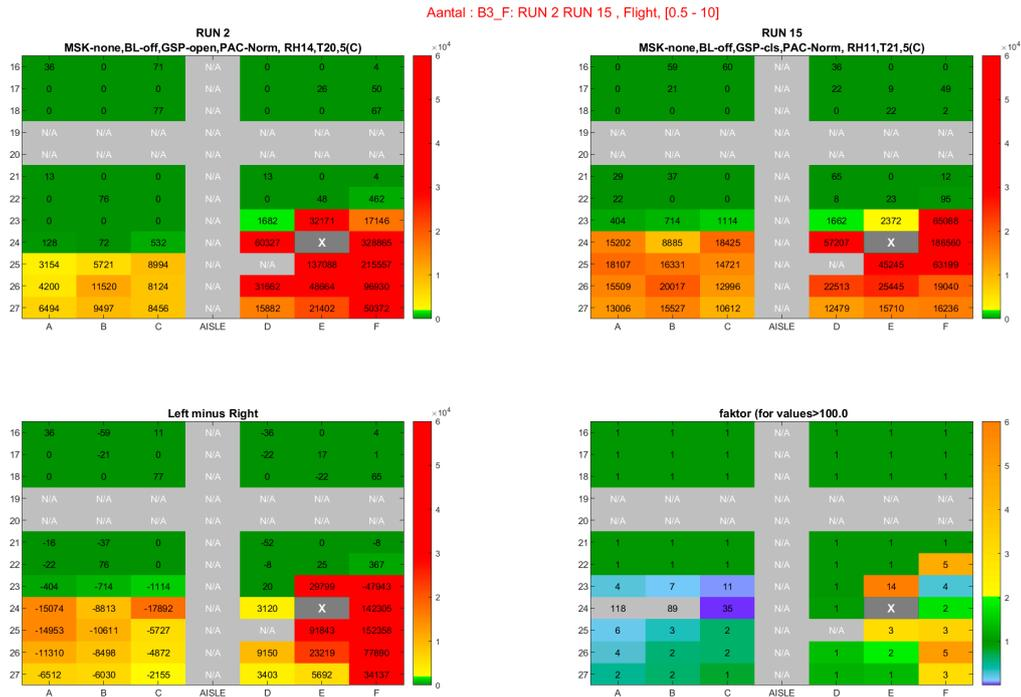
Figure 47: Aerosol distribution with gasper open (left) and gasper closed (right) in combination with no mask on index during cruise in A320
