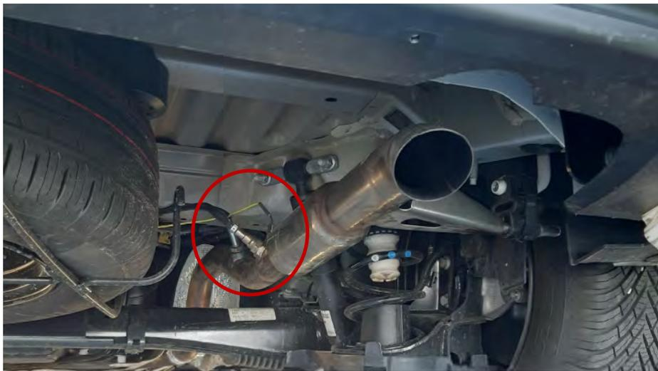
Figure 2.1: A NH<sub>3</sub>, a thermocouple and a NO<sub>x</sub> sensor installed at the end of an exhaust pipe.
