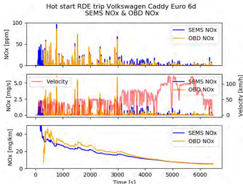
Figure 4.7: Hot start RDE trip with Volkswagen Caddy Euro 6d, SEMS NO<sub>x</sub> versus OBD NO<sub>x</sub>.
