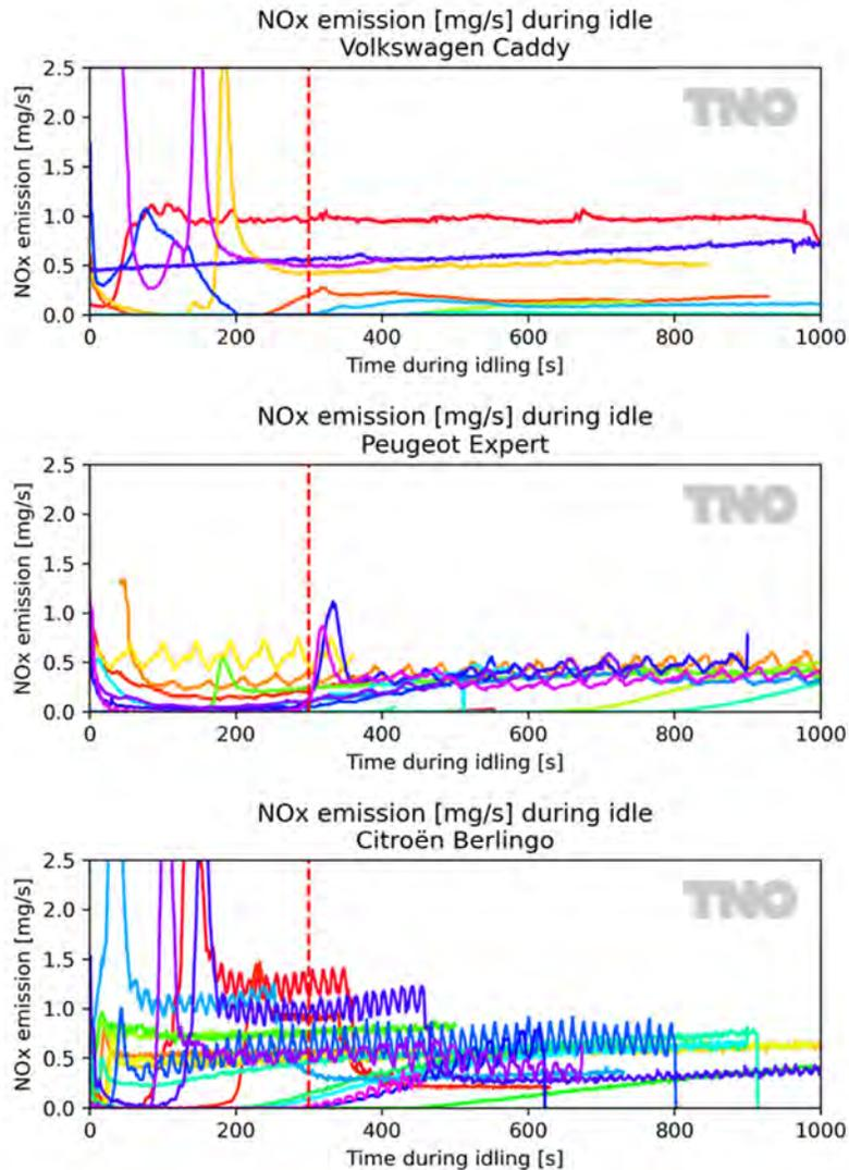
Figure 3.8: NO<sub>x</sub> emissions during (long) idle engine operation of three Euro 6d diesel vehicles. Each coloured line represents an idling session.
