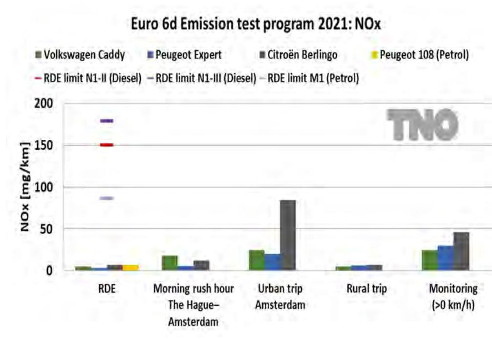
Figure 3.1: NO<sub>x</sub> emission results per test trip of the emission test program for three Euro 6d diesel vehicles and one Euro 6d petrol vehicle. The Peugeot 108 petrol was measured with PEMS and did not participate in the emission test program besides the RDE trip. The RDE trips for the diesel vehicles include a hot start and the RDE trip for the Peugeot 108 include a cold start.
