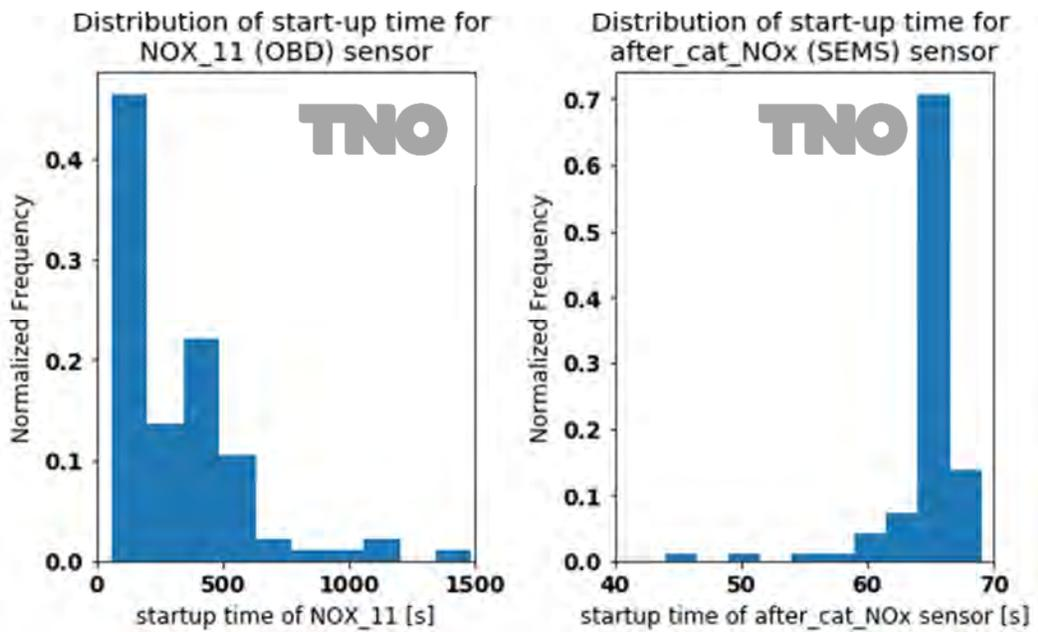
Figure 4.5: Monitoring data of the Euro 6d Citroën Berlingo. On the left: distribution of start-up times of the in-vehicle NO<sub>x</sub> sensor (pre-ASC). On the right: distribution of start-up times for the SEMS NO<sub>x</sub> sensor.
