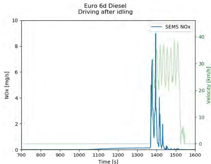
Figure 3.7: The NO<sub>x</sub> emissions increase after a period of idling. When driving after idling there is a NO<sub>x</sub> emission peak which the empty catalyst is unable to reduce.
