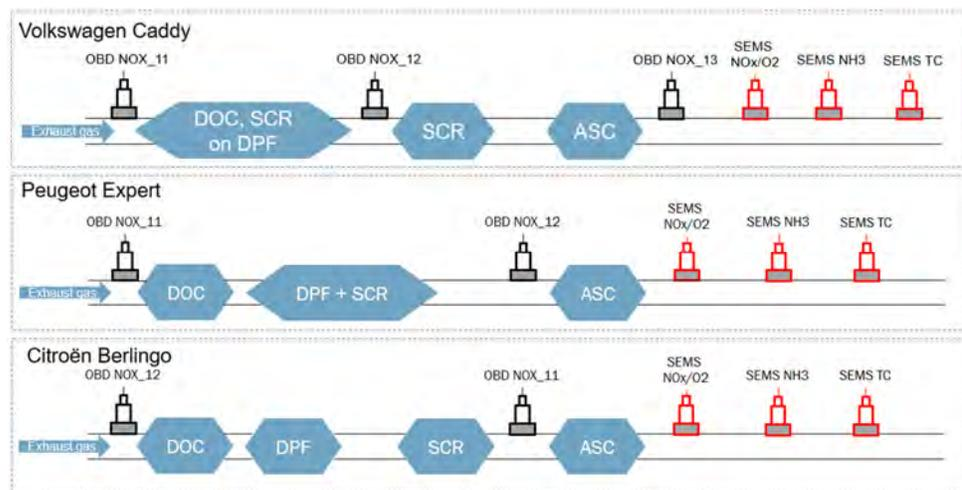
Figure 4.1: Schematic overview of the position of catalysts, in-vehicle NO<sub>x</sub> sensors and installed SEMS sensors (in red) in the exhaust pipes of the three tested Euro 6d diesel vehicles. For each vehicle the in-vehicle NO<sub>x</sub> sensors (named 'OBD NOX\_1x') have a different position in the exhaust pipe. Only the in-vehicle NO<sub>x</sub> sensor ('OBD NOX\_13') of the Volkswagen Caddy is measuring actual tailpipe-out NO<sub>x</sub> emissions.
