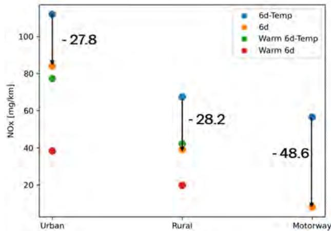
Figure 5.1: Drop in NO<sub>x</sub> emission factors from Euro 6d-Temp to 6d diesel vehicles for urban, rural and motorway segments.
