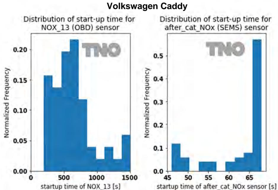
Figure 4.2: Monitoring data of the Euro 6d Volkswagen Caddy. On the left: distribution of start-up times of the in-vehicle NO<sub>x</sub> (tailpipe-out). On the right: distribution of start-up times for the SEMS NO<sub>x</sub> sensor.
