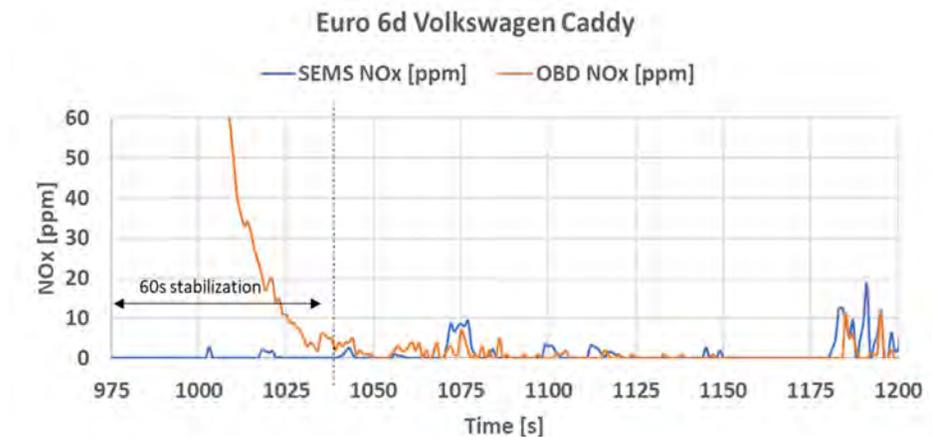
Figure 4.3: Stabilization time after activation of the OBD NO<sub>x</sub> sensor of the Euro 6d Volkswagen Caddy.
