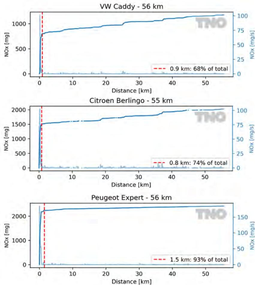
Figure 3.3: NO<sub>x</sub> emissions during a full engine load cold start trip of three diesel- and one petrol Euro 6d vehicle(s). The red dotted line indicates the point where the exhaust aftertreatment system is working well. These cold start distances show that in the first few hundred meters more than 68% of the total trip NO<sub>x</sub> emissions are emitted for the three diesel vehicles.
