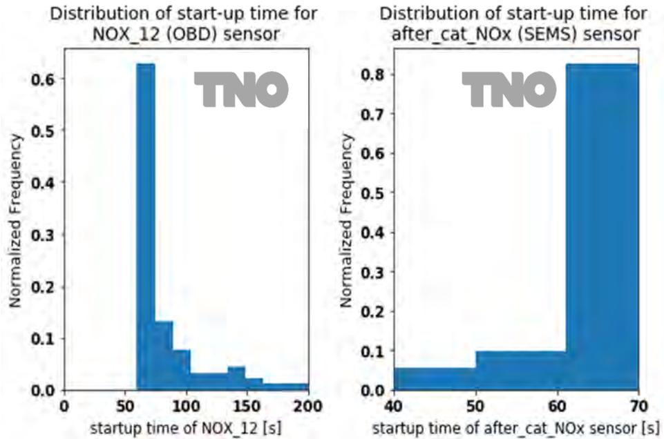
Figure 4.4: Monitoring data of the Euro 6d Peugeot Expert. On the left: distribution of start-up times of the in-vehicle NO<sub>x</sub> sensor (pre-ASC). On the right: distribution of start-up times for the SEMS NO<sub>x</sub> sensor.
