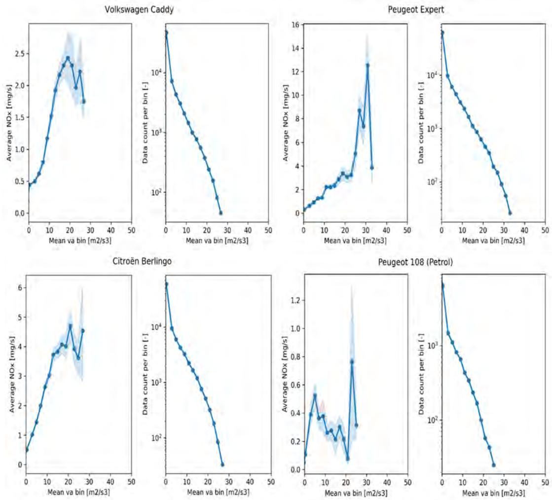
Figure 3.10: Relation between dynamic driving and average NO<sub>x</sub> emissions for three Euro 6d diesel vehicles and one petrol vehicle.
