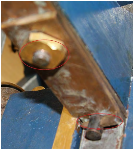
The lower fuse of the bolt was widely used until the first half of the 18th century. The copper flat nut is not; presumably this is a later restoration? (Rijksmuseum, Amsterdam, Behandelingsrapport NG-NM-1015, 2012)
