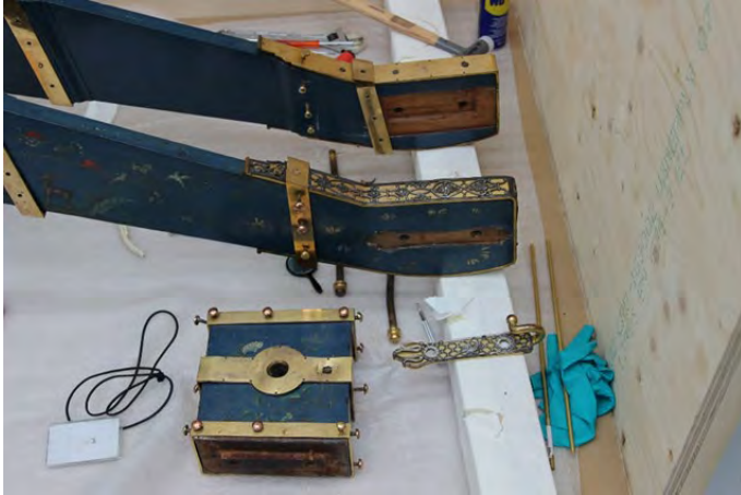
The wooden tailstock with the drawbar eye is very shallowly recessed between the two sides and the copper bolts are very thin.
