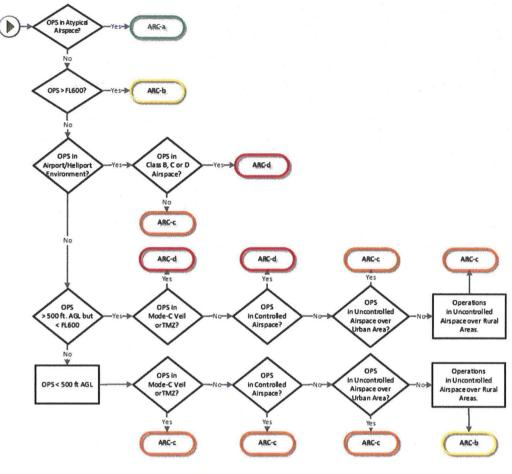
Figure 3 Flowchart ARC determination
