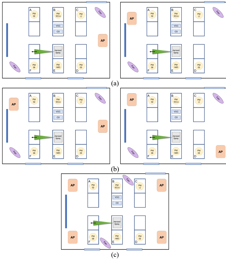
Figure 6. Configuration of the mobile air cleaning devices in the Experience Room. (a) One unit: left – C1, right – C2. (b) Two units: left – C1, right – C2. (c) Four units: C1.
