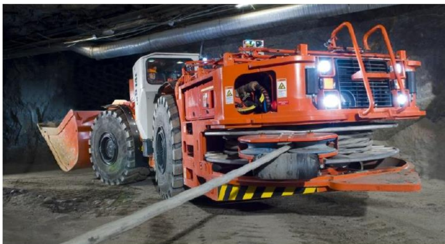
Figure 3: Example of NRMM without on-board power source: a wheel loader used in mining
