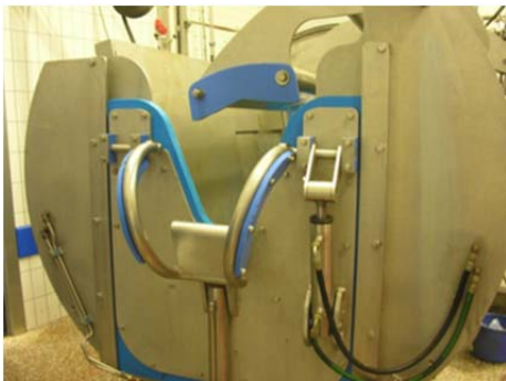
Figure 4: example of a NAWI restrainer for cattle in a slaughter plant
