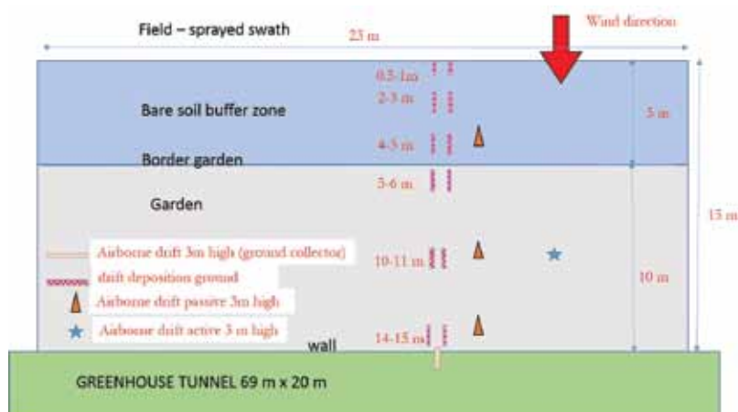
Figure 5.5: Schematic overview of the collector positions in different collector arrays, garden border and (green) house wall per measuring object.
