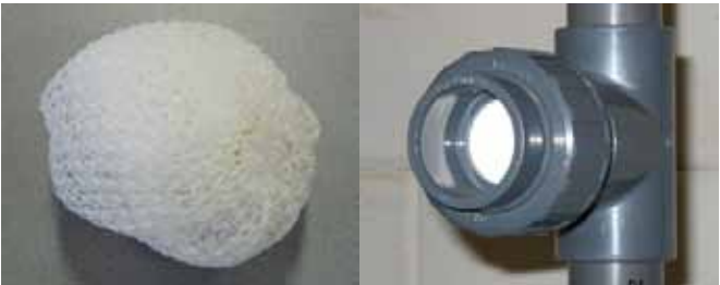
Figure 5.1: Passive collector (left) and active collector in suction head (right) for measuring airborne spray drift.
