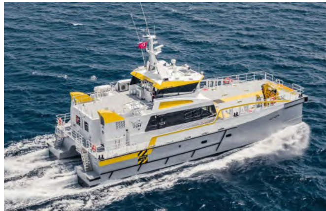
Crew transfer vessel. Photo: © Damen.
