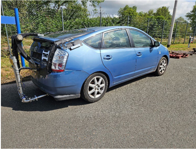
Figure 3.1: The Toyota Prius test vehicle equipped with PEMS test equipment ready for on-road testing
