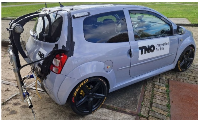
Figure 4.1: Renault Twingo instrumented with a PEMS system undergoing stationary testing with an additional 5-gas analyser (PTI 4-gas analyser + \text{NO}_x ) sampling in the exhaust tip.
