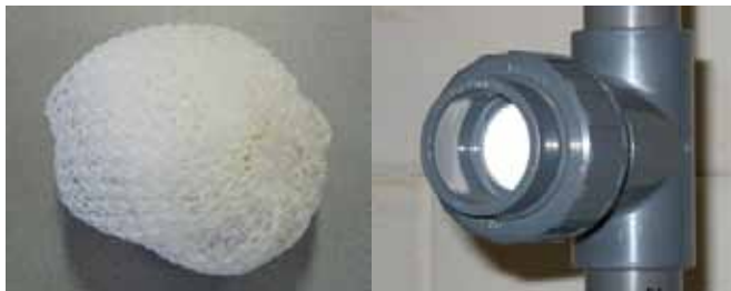
Figure 5.1: Passive collector (left) and active collector in suction head (right) for measuring airborne spray drift.
