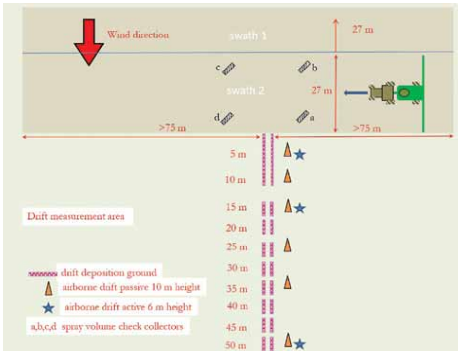
Figure 5.7: Schematic presentation of the spray drift collector setup in the downwind drift measurement area and the treated area (swath 1 + swath 2 and on top of crop canopy (a, b, c, d) to check applied spray volume) at the experimental field.
