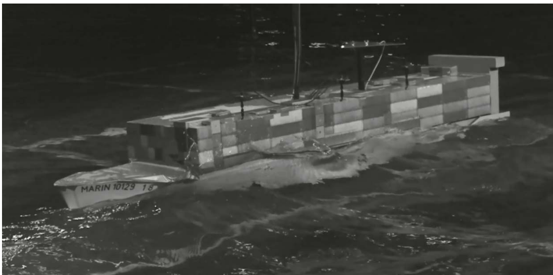
Green water loading on the Feeder (Hs = 4.5 m, Tp = 10.2 s, Vs = 0 kn)
