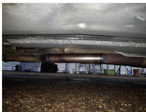
Catalytic converter replaced by a straight exhaust pipe, German BMW from 2001 (left picture) and a German Mercedes C180 from 2000 (right picture) © ILT December 2019
