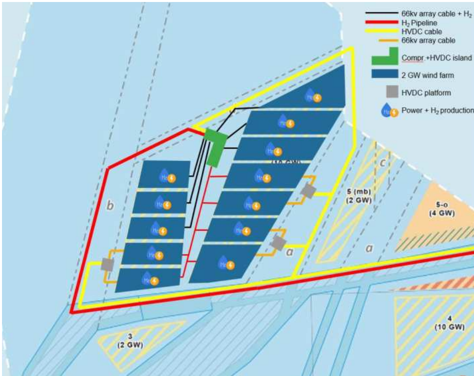
Figure 3.7: Illustrative Layout of Concept 3 – Platform-based Hub but with Centralised Compression on an Island with 6 GW of HVDC Equipment
