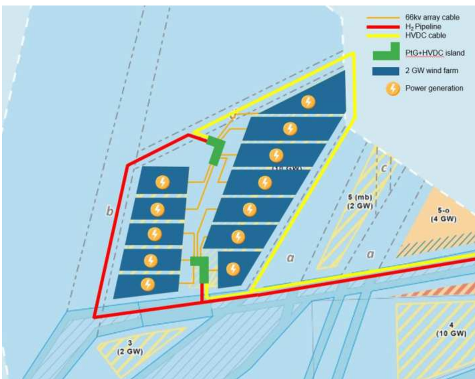
Figure 6.19: Illustrative Layout of Concept 1 – Large Island supporting Hydrogen Production.
