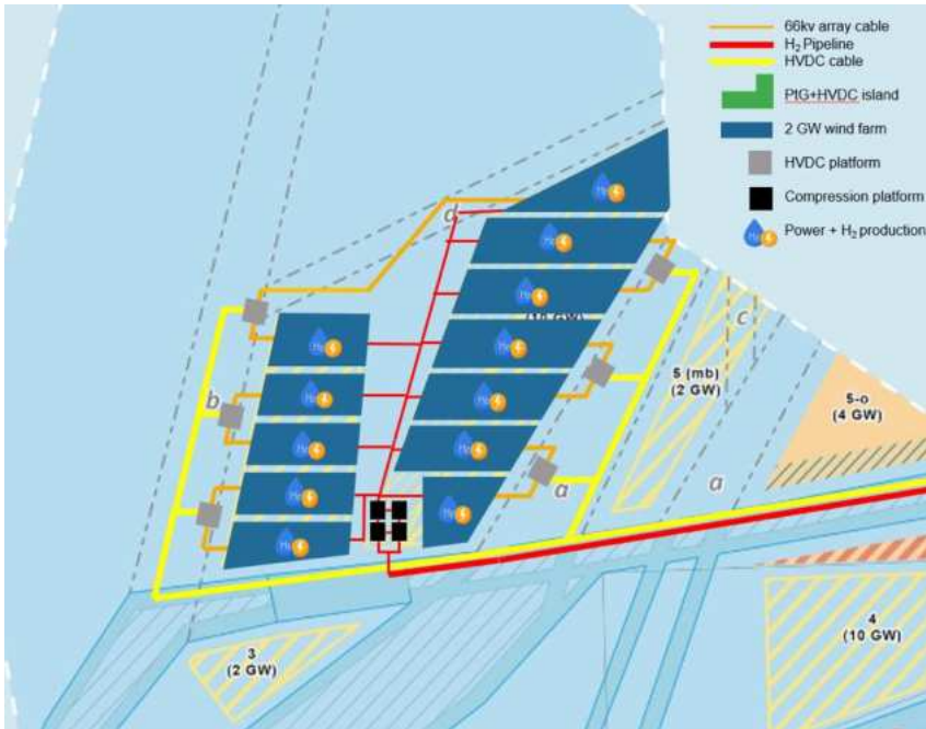
Figure 6.5: Illustrative Layout of Platform-based Energy Hub (concept 2a).
