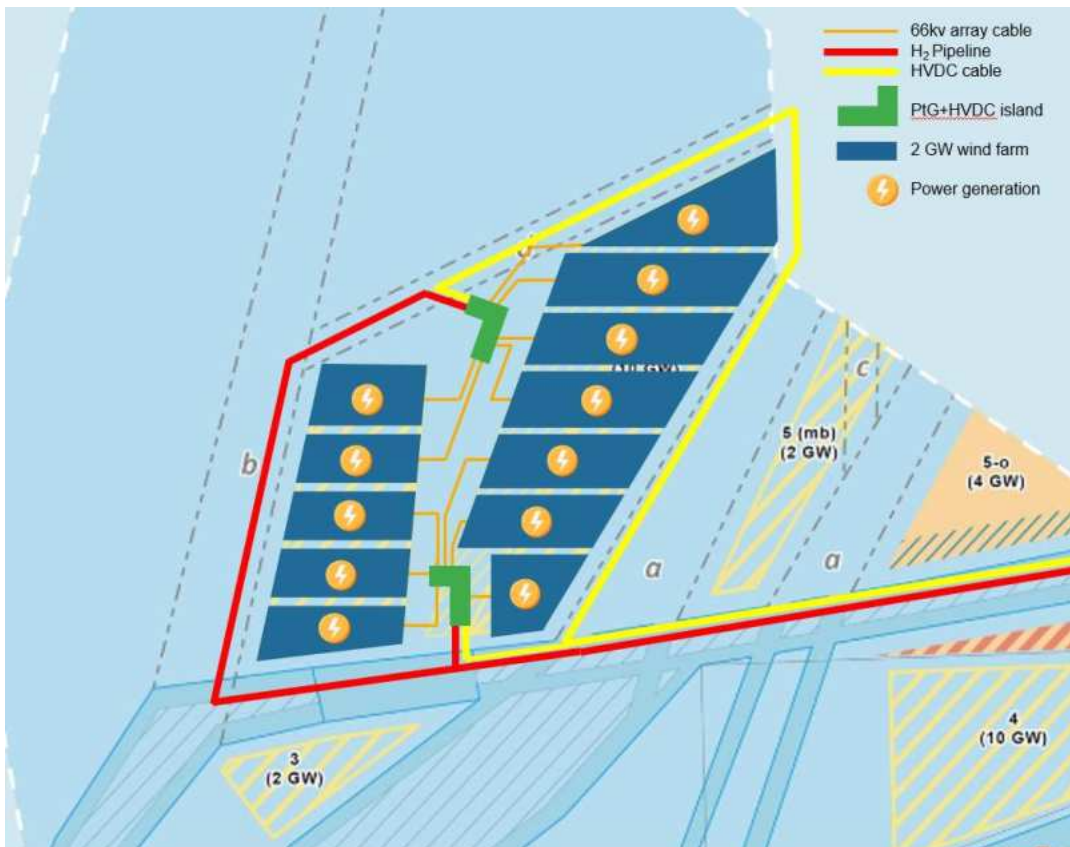
Figure 3.4: Illustrative Layout of Concept 1 – Large Islands supporting hydrogen production.
