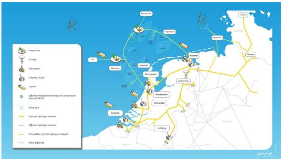
Figure 2.7: Illustrative Offshore Hydrogen Network of HyNetwork Services (ref. 31).
