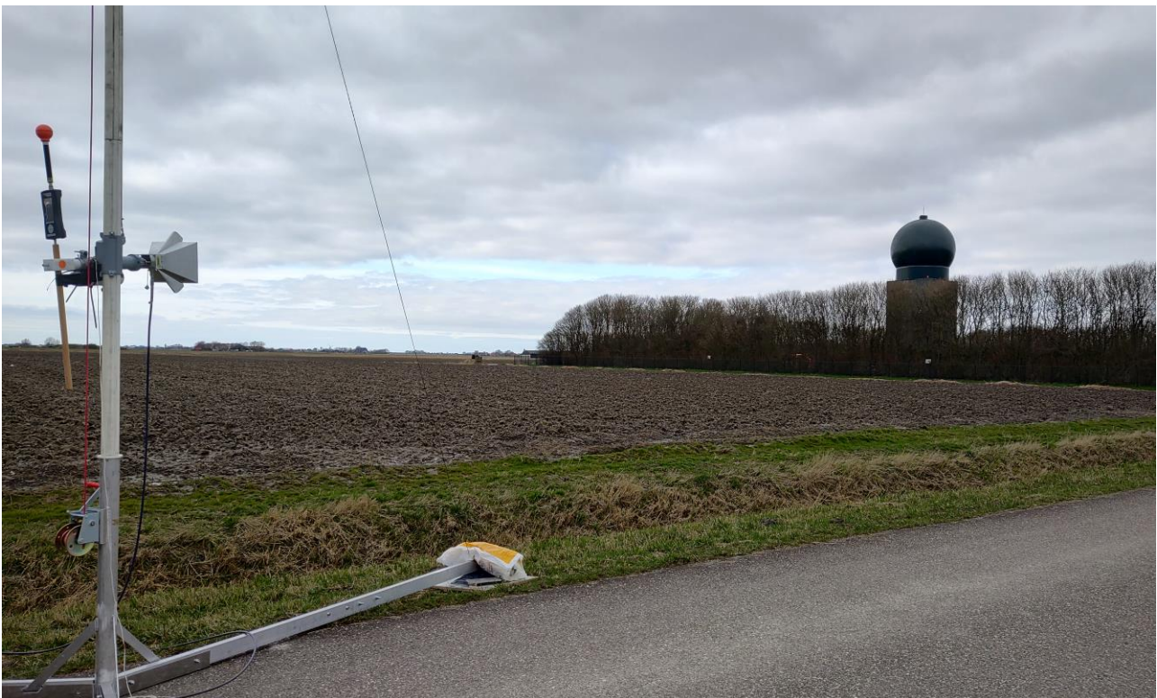
This photo shows measurements using horn antenna and hand-held meter while the antenna and the hand-held meter are position at 2 m. height above the ground.
