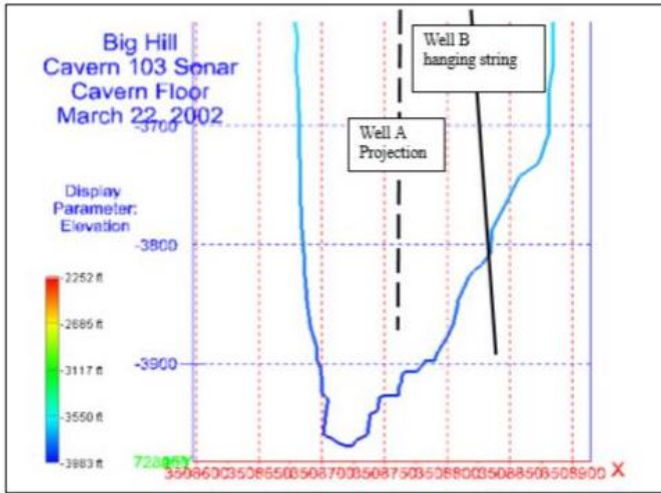
Figure 111. The Well B hanging string is buried in debris that accumulated on the east wall (Munson et al., 2004).
