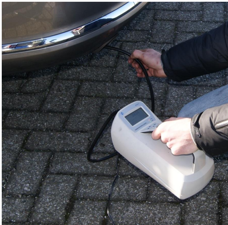
Figure 5 The particle number (PN) measurements were performed using the TSI 3007, a handheld Condensation Particle Counter (CPC). A sample hose, connected to the 3007, was kept in the exhaust flow with the engine running at idle engine speed.
