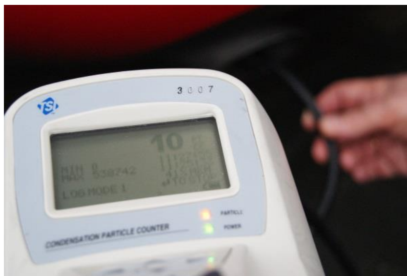
Figure 6 The sample hose was kept in the exhaust pipe until the read-out stabilized.
