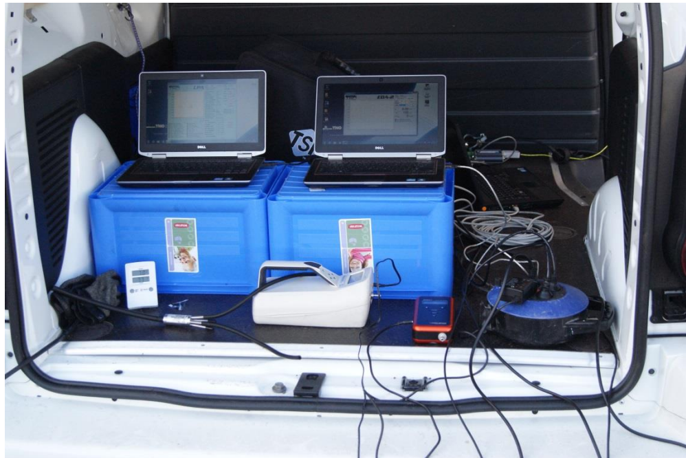
Figure 7 The smoke meters were connected to a laptop and data was logged using dedicated software. The TSI 3007 logs data internally, and test data was retrieved from the device by connecting it to a laptop at the end of a measurement day.
