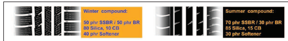
Figure 3.1: Comparison of typical winter and Summer tyre [8].
