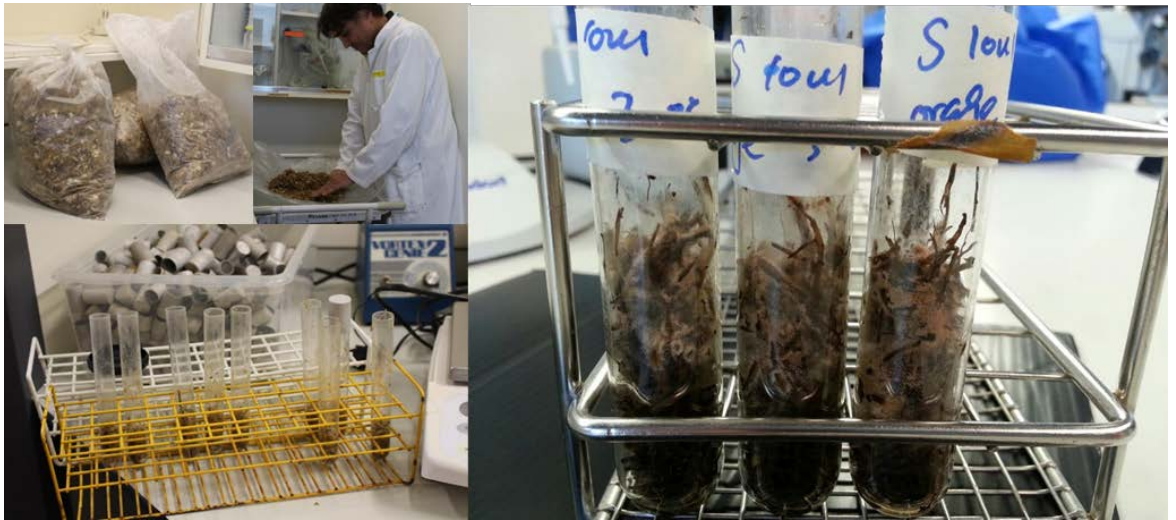
Figure 7. Pictures of the experimental laboratory hotspot model. Each glass tube is filled with decaying plant material, azole fungicides (or not) are added and fungal inoculum. Tubes are incubated at 37 °C
