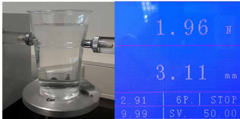
Figure 39: Cup Compression Tests instrumentation
