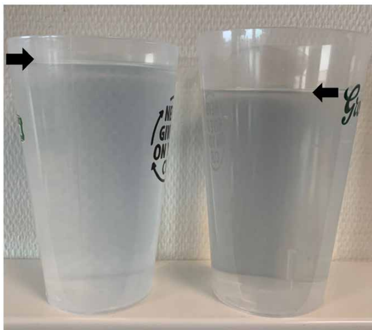
Figure 38: The 200 and 250 ml (H)PP 1 Hard Cups filled with 250 ml of water
