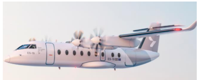
Figure 7 - Heart Aerospace ES-19, all-electric 19-seats aircraft (source: Heart Aerospace)
