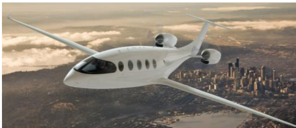
Figure 6 - Eviation Alice, all-electric 9-seats aircraft (source: Eviation)
