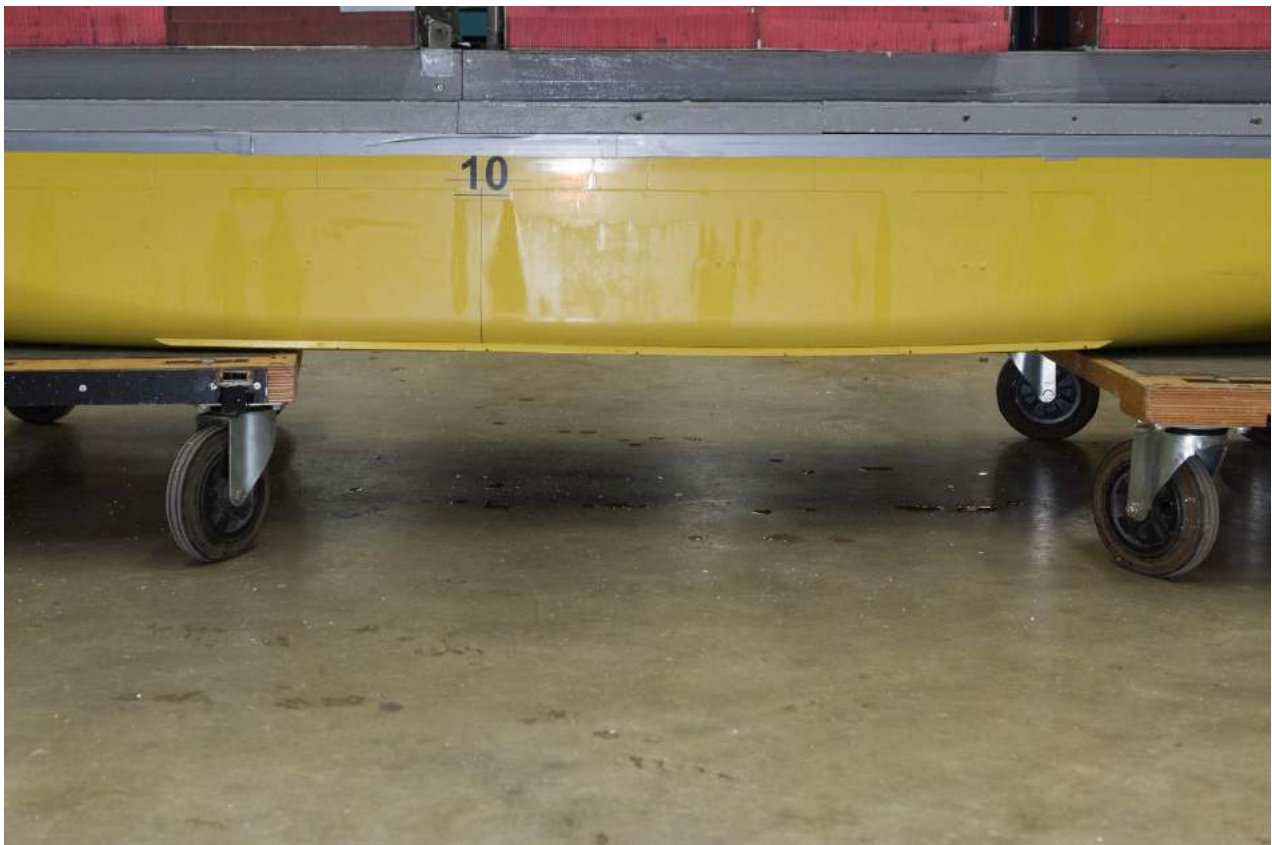
Photo 8 Details of the bilge keels – LC 2
