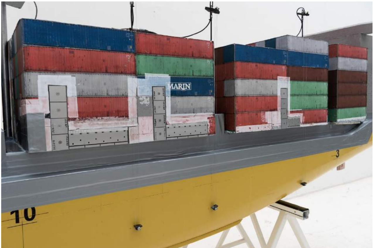
Photo 12 Details of the force panels
