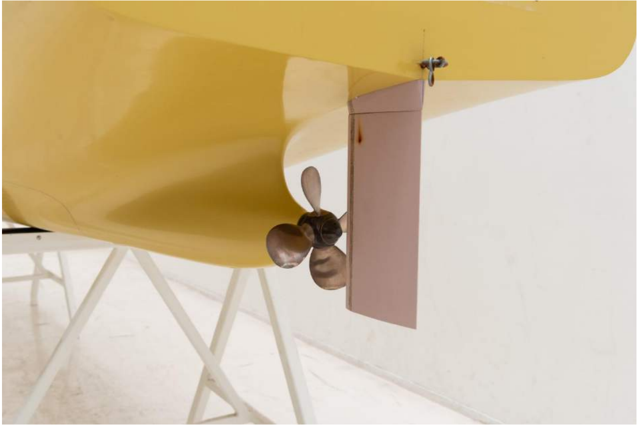
Photo 6 Details of the rudders and propellers
