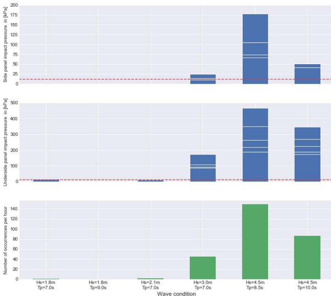
Figure 3-20: Stacked-up representation of the top five transverse wave load pressures (top), top five vertical wave load pressures (middle) and hourly number of occurrences (bottom) Different wave conditions, heading 270 deg, depth 21.3 m, short-crested waves
