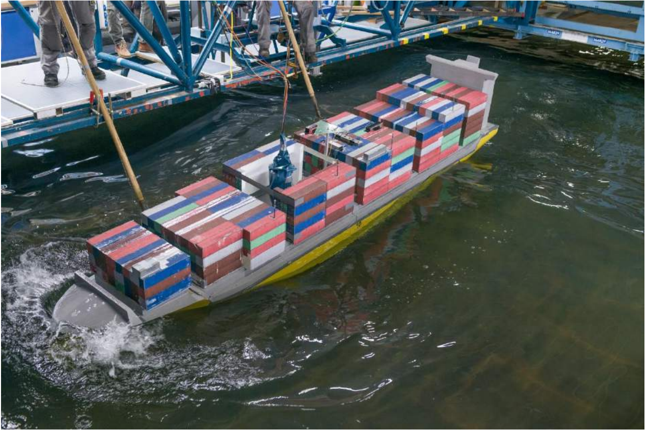
Photo 16 Test 33327_02BT_04_001: \mu = 180 deg – H_s = 6.0 m – T_p = 11.8 s – V_s = 4 kn
