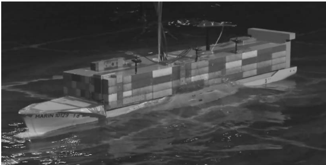
Figure 1-1: Green water loading on the lowest tiers of deck containers on a feeder ship, MARIN report 32558-2-OB
