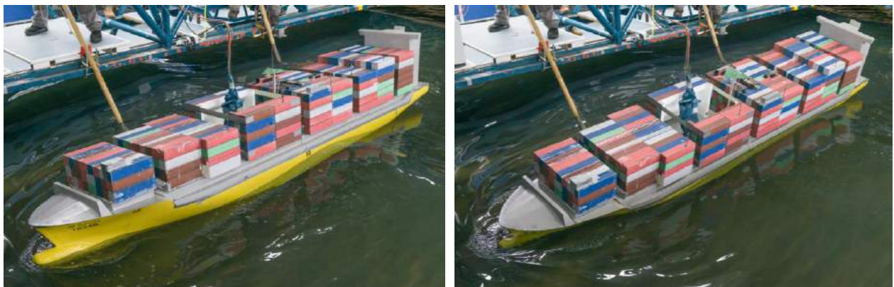
Figure 3-41: Occurrence of parametric roll during the test in head waves - Hs = 6 m, Tp = 11 s
