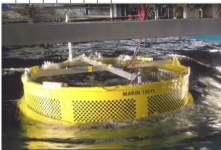
Extreme event matching applied to obtain local pressure distributions during internal sloshing inside a floating fish farm (courtesy of Viewpoint Seafarm AS - Spider Cage concept).
