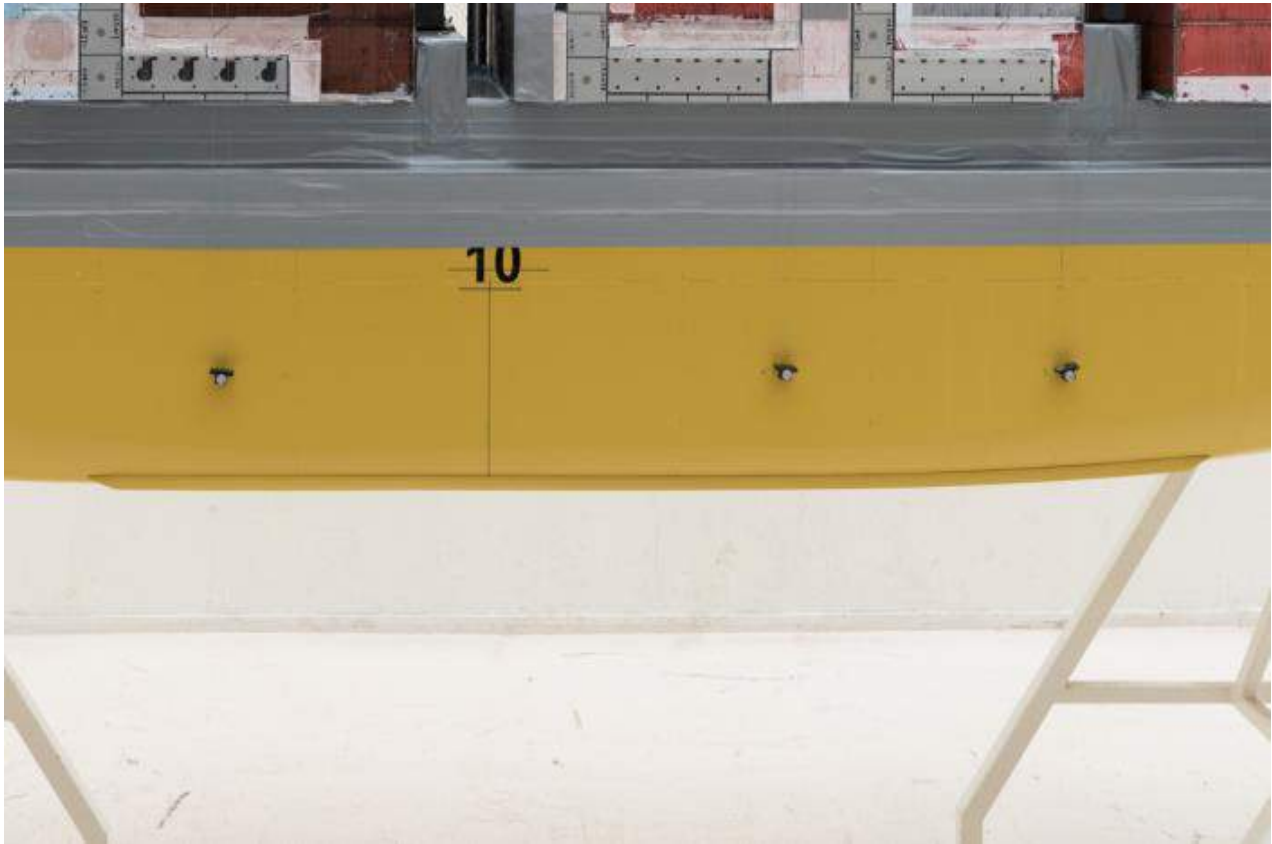
Photo 8 Details of the bilge keels – LC 2
