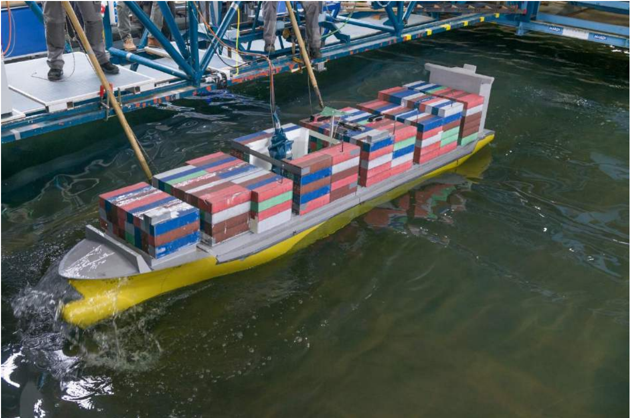
Photo 16 Test 33327_02BT_04_001: \mu = 180 deg – H_s = 6.0 m – T_p = 11.8 s – V_s = 4 kn
