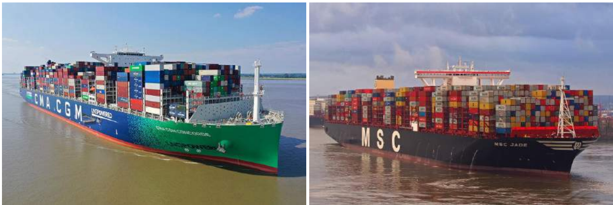
Figure 5-1: Examples of ULCS containerships. To the left a modern bow shaped 62 m width ULCS. To the right a more typical bow shaped ULCS (59 m beam).
