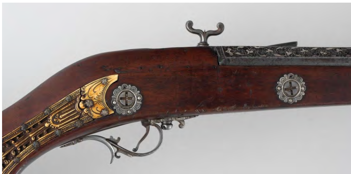
Photo 4: Metropolitan Museum of Art in New York, Inventory Number: 91.1.907, Dating: 1680AD, Two Crosshead screws in the gun stock
