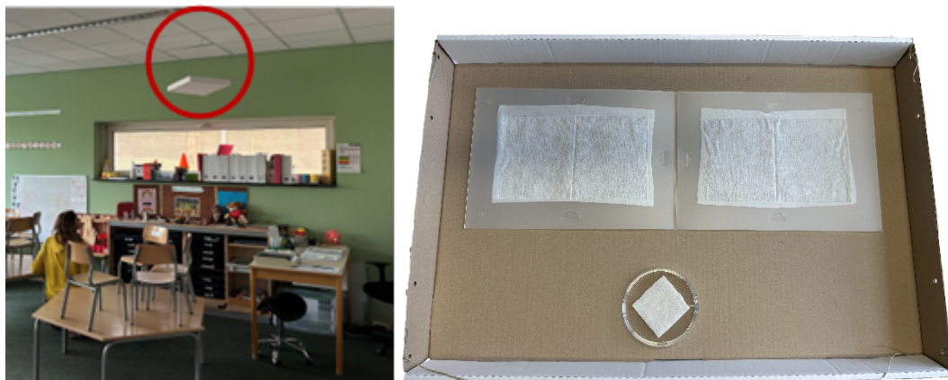
Figure F1: Left; a sampler box (in red circle) hanging in a classroom Right; interior view of a cardboard box used for sampling containing an EDC (top) and a mini-EDC (bottom).
